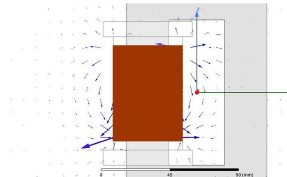
Fig.6 Electric field around the secondary winding in electrostatic simulation.
