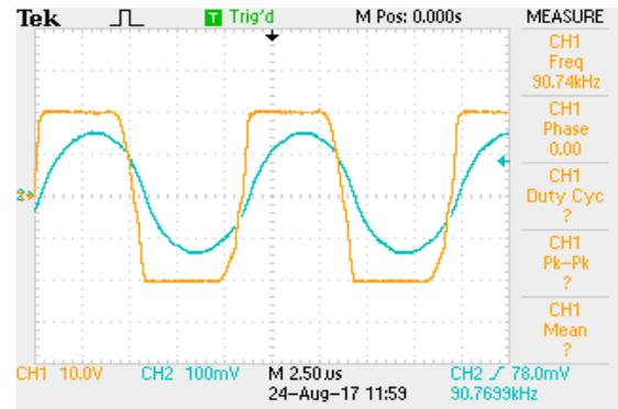
Fig.8 experimental results: Compared inverter voltage and resonant tank current
