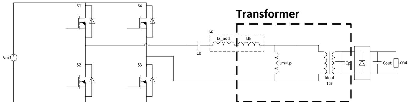
Fig.3 LCLC Resonant Converter
