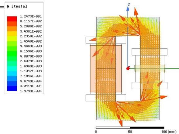
Fig.5. Flux density through the core by magnetostatic simulation
