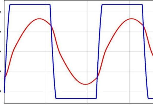
Fig.7 Simulation results: Inverter voltage vs. resonant tank current
