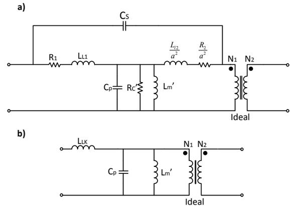
Fig.1 a) Detailed model b) Proposed model for high voltage transformer
