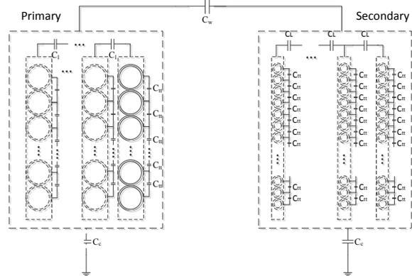
Fig.2 Parasitic capacitances in transformer
